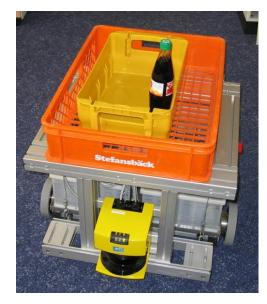
Use of a planar laser scanner for obstacle detection and position determination
